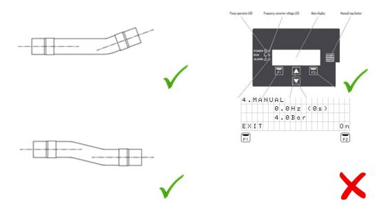
We supply various size flexible connections from 1 1/4" to 4" to suit our manifold sizes. The smaller sizes are more pliable but still should not be used as elbows. The bigger sizes are very rigid and may not bend very easily. As with any flexible connector, if they are overly bent through awkward angles they will kink and become unusable, as the bore will be reduced and may not allow the required amount of flow through the pumps or to the system.
