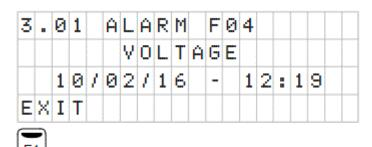
Use the arrows to move forward or back to view the different alarms that have been triggered. Press F1 to exit this menu.
