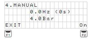
The display will show the frequency, an operation timer and the pressure at that precise moment read by the transducer.
