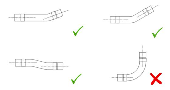
We supply various size flexible connections from 1 1/4" to 4" to suit our manifold sizes. The smaller sizes are more pliable but still should not be used as elbows. The bigger sizes are very rigid and may not bend very easily. As with any flexible connector, if they are overly bent through awkward angles they will kink and become unusable, as the bore will be reduced and may not allow the required amount of flow through the pumps or to the system.
