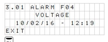
Use the arrows to move forward or back to view the different alarms that have been triggered. Press F1 to exit this menu.
